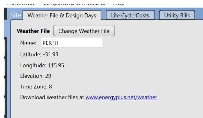
Figure 3. A weather file for Perth, WA, Australia was downloaded from www.energyplus.net/weather and imported on the Open Studio software.
